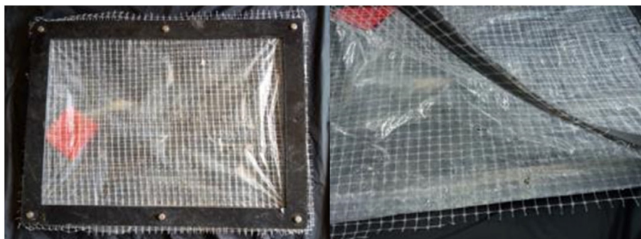
Fig. 2. Sample supporting system consisting of a rigid frame and plastic net with mesh size 7 × 7 mm.
