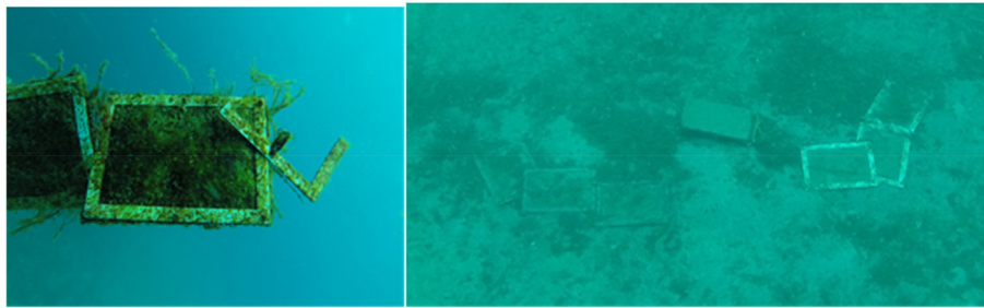
Fig. 18. Samples exposed to the pelagic environment were destroyed during the 2nd year due to storms (PHB samples were lost). Samples exposed to the benthic environment were displaced along with their anchor several meters from their initial position by forces applied by the waves through the buoys and water currents.
